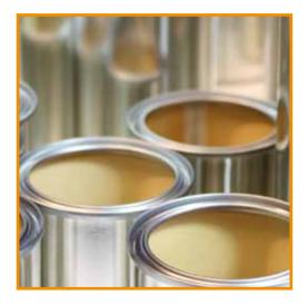
Cylindrical tinplate cans are the classic packaging for paint, lacquer and wood-stains. The shape is round, the body is straight (so it cannot be stacked) and there is a ring at the top in which the lid closes. The ring can be RL shaped (lid closes on the inside of the ring) or TT shaped (lid falls inside the ring and closes at three places as it were).
