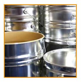
Pails are all tinplate packaging with a capacity of 10 to 30 litre. Within this category there is a distinction between the various diameters. The 286 mm, 305 mm and 328 mm diameters are the most common. The height of the pail in combination with the diameter determines the container's capacity. All pails are constructed out of tinned plate steel. Pails always have a handle because of their large size, and conical in shape.
